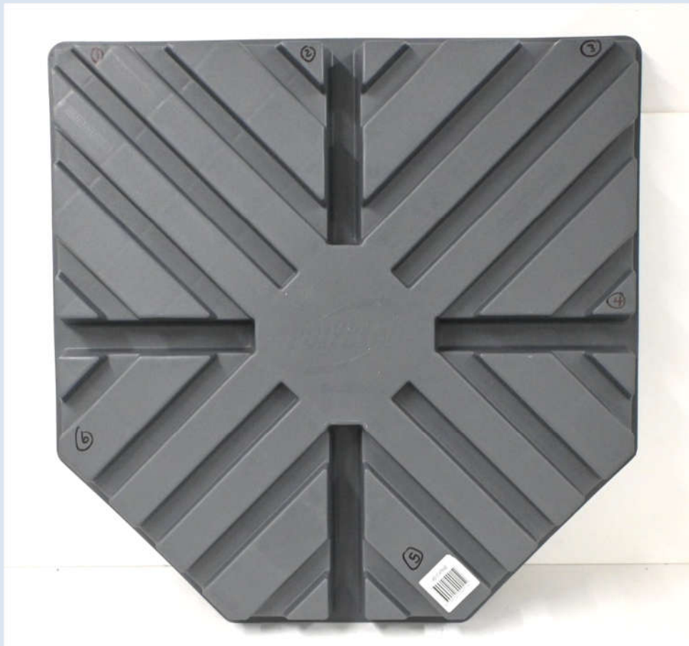
Figure 4.1 – Hot water service base, top view, marked with thickness assessment locations
