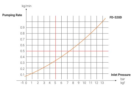
Note: The gas pumping rate is proportional to the inlet pressure.
